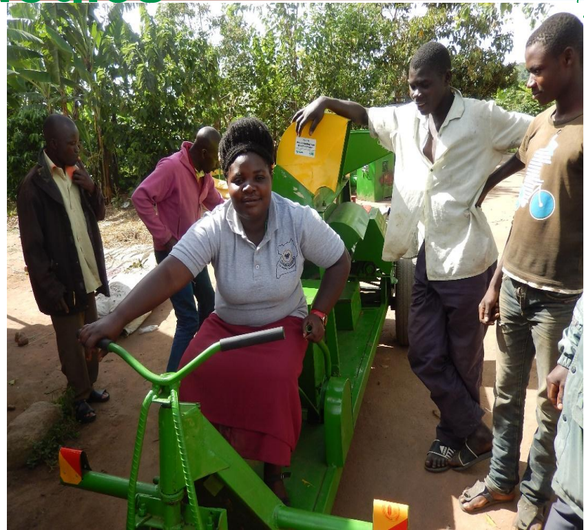
Combined Mobile Bean Thresher with a mobile irrigation pump
